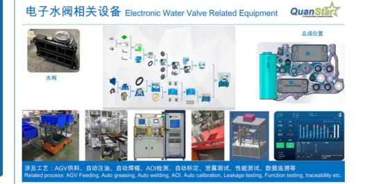
The design of the assembly line for electric vehicle electronic water valve focuses on flexibility and high efficiency. Feeding: Set up sensors and visual recognition systems at the feeding position to quickly identify and classify parts to ensure the accuracy of parts by identifying the QR code or specific mark of parts, automatically distribute valve bodies, valve cores and other parts of different specifications to the corresponding assembly stations.
